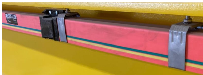
2.1.3 ElectroTrack Hanger Bolted Directly to I-Beam
