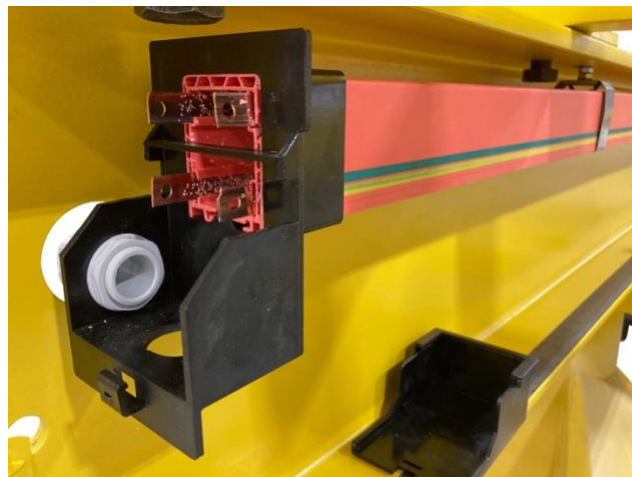
2.3.1 End of ElectroTrack System
